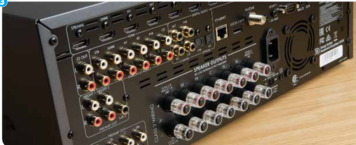
3. The AVR390 has no analogue video inputs at all. It's HDMI or bust
